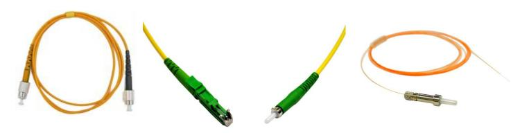
Thermally expanded core termination is used to ease coupling between fiber and free space. Core thermal expansion allows coupling beams with higher mode field diameter and numerical aperture to the standard single mode fiber. The terminations are available as patchcords with connectors, patchcords with connector and ferrule (TEC side) or as pigtails with a ferrule on the TEC side.
